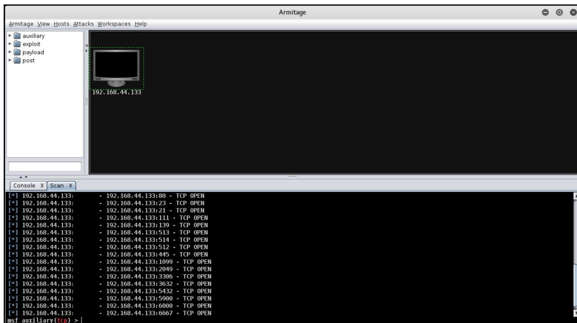
As we have seen earlier, Armitage is also well-integrated with NMAP. Now, we'll perform an NMAP scan on our target to enumerate services and detect the version of the remote operating system, as shown in the following screenshot. To initiate the NMAP scan, click on the **Hosts** option, select the **NMAP** scan, and then select the **Quick Scan (OS Detect)** option:
